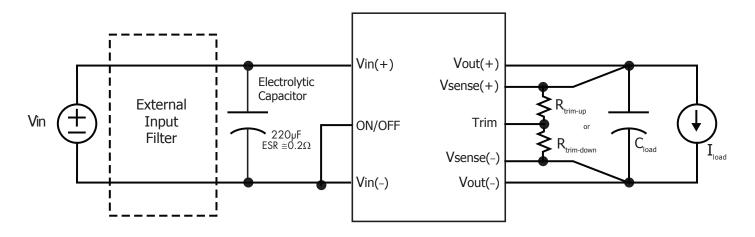
Figure E: Typical application circuit (negative logic unit, permanently enabled).
