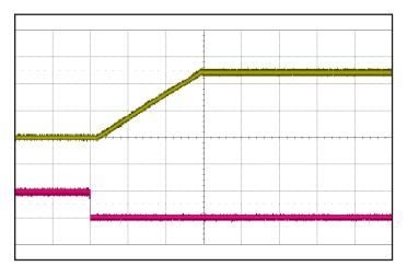
Figure 6: Turn-on transient at zero load (10 ms/div).
