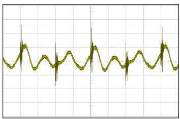
Figure 12: Output voltage ripple at nominal input voltage and rated load current (50 mV/div; 2  $\mu$ s/div). Load capacitance: 1  $\mu$ F ceramic capacitor and 15  $\mu$ F tantalum capacitor. Bandwidth: 20 MHz. See Figure 9.
