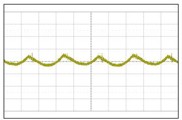
Figure 10: Input Terminal Ripple Current, ic, at full rated output current and nominal input voltage with 4.7 µH source impedance and 220 µF electrolytic capacitor (1 A/div; 2 µs/div). See Figure 9.
