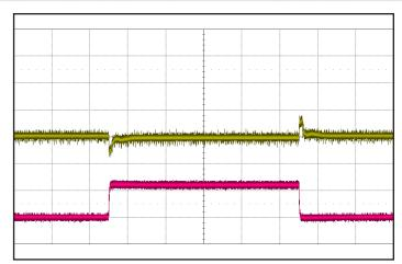
Figure 7: Output voltage response to step-change in load current (50%-75%-50% of lout(max);  $dI/dt = 0.1 \ A/\mu \ s$ ;  $1 \ ms/div$ ). Load cap:  $1 \ uF$  ceramic and 470  $\mu F$  electrolitic capacitors. Top trace: Vout (500 mV/div). Bottom trace: lout (10 A/div).
