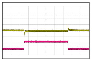
Figure 8: Output voltage response to step-change in load current (50%-75%-50% of lout(max):  $dI/dt = 5 A/\mu s$ ; 1 ms/div). Load cap: 470  $\mu$ F electrolitic capacitor. Top trace: Vout (500 mV/div). Bottom trace: lout (10 A/div).
