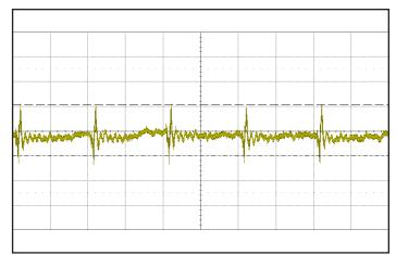
Figure 11: Input reflected ripple current, is, through a 4.7 µH source inductor, using a 220 µF input capacitor, at nominal input voltage and rated load current (10 mA/div; 2 µs/div). See Figure 9.
